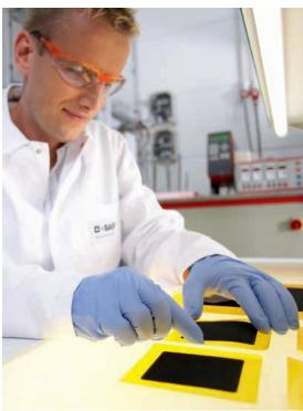
The Celtec® membrane is the core of high-temperature membrane electrode assemblies (MEA) that can be used for fuel cells and electrochemical hydrogen separation. This MEA operates at temperatures between 120 and 180 °C, tolerates large concentrations of carbon monoxide and is capable of running independently of humidification. This technology enables fuel cell systems to become simpler and more cost effective.
